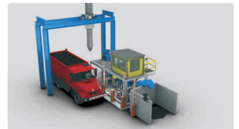
Sample extraction from the trucks or railway wagons using the auger sampler mounted on the gantry positioning device
